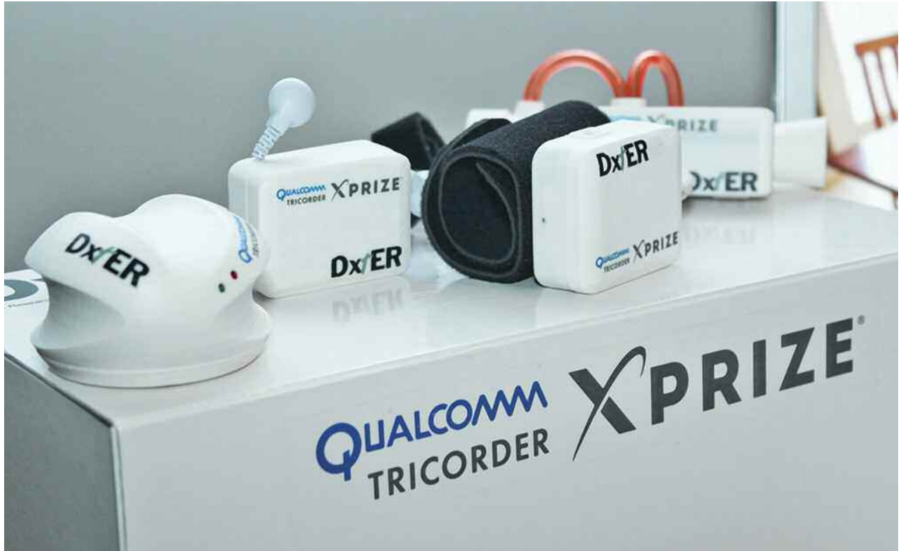
DxtER, similar to the “Star Trek” tricorder seen in the 1960s television series, is a handheld device that helps doctors diagnose patients based on symptoms. It won the top prize at the Qualcomm Tricorder XPRIZE competition.
